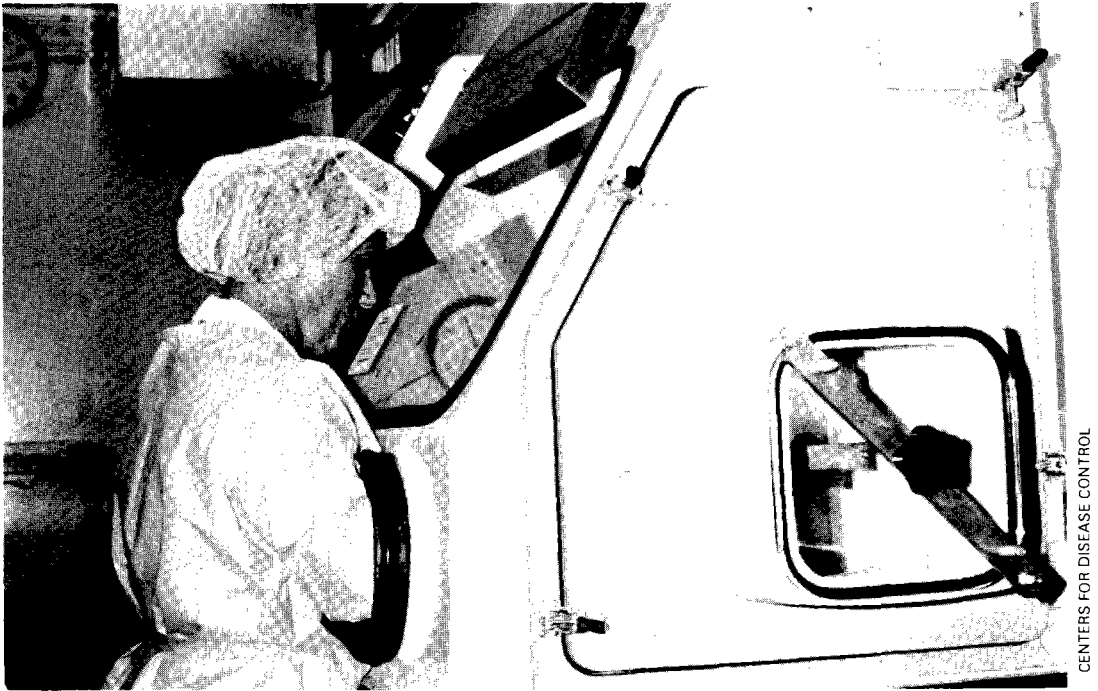
Plate 30.3. Glovebox facility (Class III biological safety cabinet) in use at the WHO collaborating centre in the Centers for Disease Control, Atlanta, GA, USA. To eliminate the risk of laboratory contamination, only a single specimen was handled at a time and the cabinet was sterilized with peracetic acid before another specimen was introduced.
